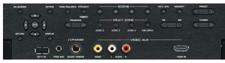
Oil-Damped Hidden Control Panel Includes HDMI Input Terminal, USB Port, Video Aux Input Terminals, Zone 2/3/4 Switch, YPAO Microphone Jack, And More.
